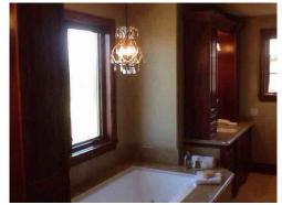
**223:** - The light fixtures pictured, appear to be somewhat larger than typical and thus, may weigh much. The junction box is suggested to be verified to withstand the weight of the light fixture. The weight limit of junction boxes is limited to 50 pounds.
