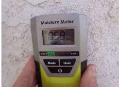
**66:** - Moisture was observed throughout the stucco covering under the south side and north side decks as well as the wall under the south side deck. The moisture appears to derive from the deck surfaces, however, a water test is suggested to be performed to confirm this.
